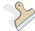
Steel rule/spatula (for support when trimming the wallpaper at ceiling and floor level)
